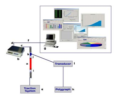
FIGURE 1 - Schematic representation of ETR. a) descendent colon segment, b) precision balance, c) strength cell, d) serial port, e) traction system, f) serial communication cable and SABI 2.0, g) computer with serial interface and SABI 2.0, h) polygraph, i) catheter cannon (closed light), j) catheter cannon (open light), k) triple-via plug attached to the supporter and l) polygraph transducer
